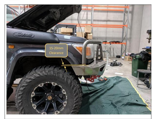
20. With assistance from another person, Align the bar with the edges of the vehicle. Adjust such that the clearances are neat and even side to side.
